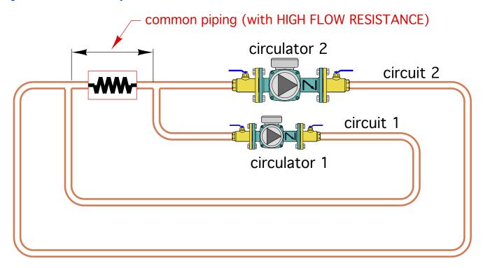
The higher the flow resistance of the common piping, the more each circulator will "influence" flow in the other circuit (e.g. the lower the hydraulic separation of the circuits).
