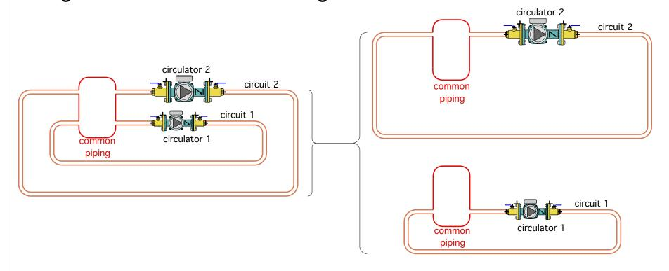
Design tip: Hydraulic separation allows designers to think of an overall system as a collection of independent ("hydraulically isolated) circuits.
