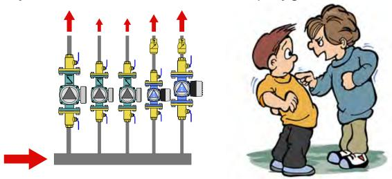
When 2 or more circulators are operating simultaneously in the same piping assembly, they try to "interfere" with each other.
