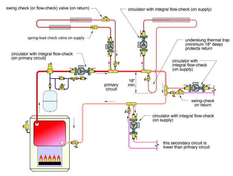
This is a SERIES primary loop. It will create a sequential drop in water temperature from one secondary circuit to the next.
