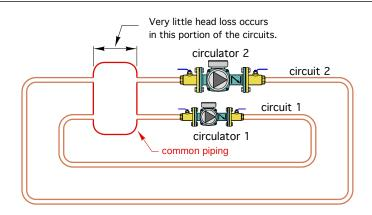
Assume that circulator 1 is operating, but that circulator 2 is off. The lower (blue) system head loss curve in figure 2 applies to this situation.
