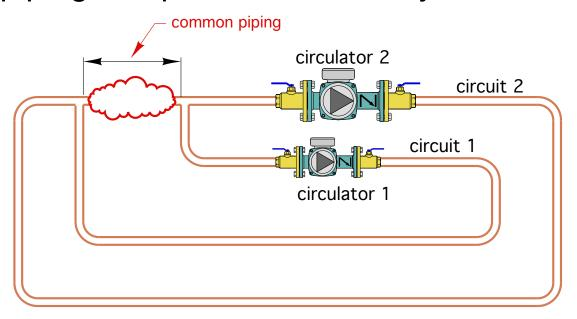
The degree to which two or more operating circulators interact with each other depends on the head loss of the common piping.
