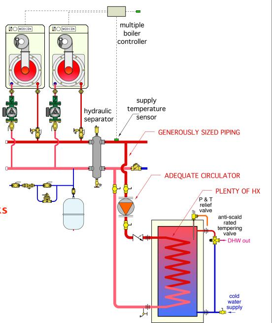
No Bottlenecks: When an indirect tank simply can't provide the necessary heat transfer, use a generously sized stainless steel flat plate heat exchanger with a standard storage
