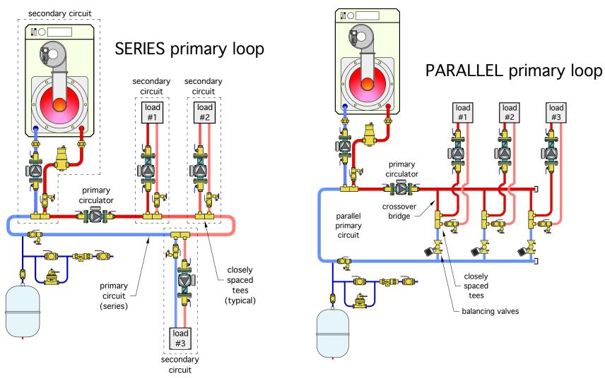
Both series and parallel primary/secondary systems require a primary circulator.
