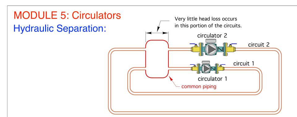
Imagine a hypothetical situation in which the head loss across the common piping was *zero*, even with both circuits operating.
