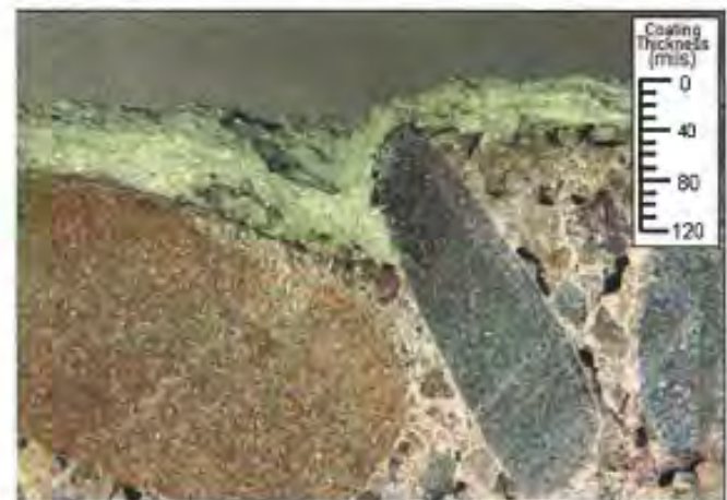
Vulcanized Latex at 40 mil dry thickness on concrete block
