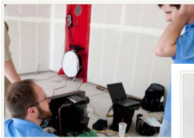
Connecting controls for blower door, setting up compressor for aerosol injection and monitoring software.
