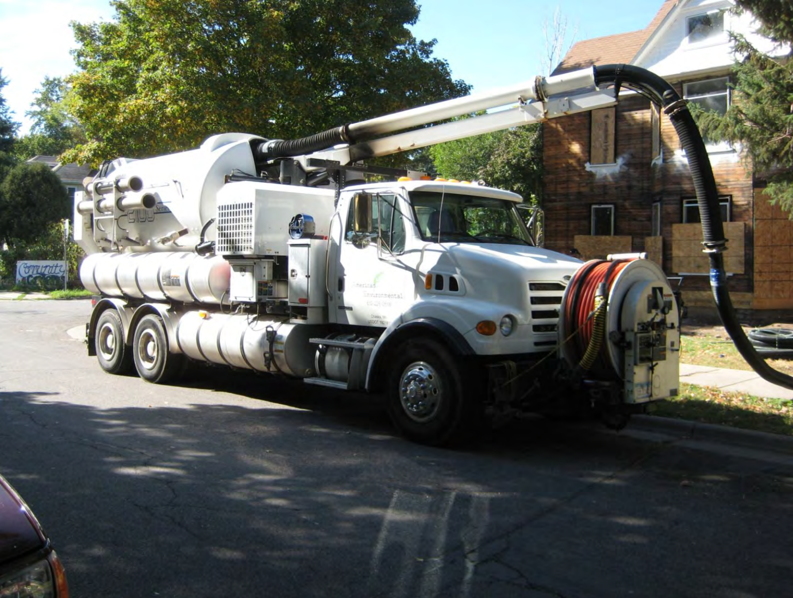
Vacuum excavator truck, American Environmental, 12 yard capacity
