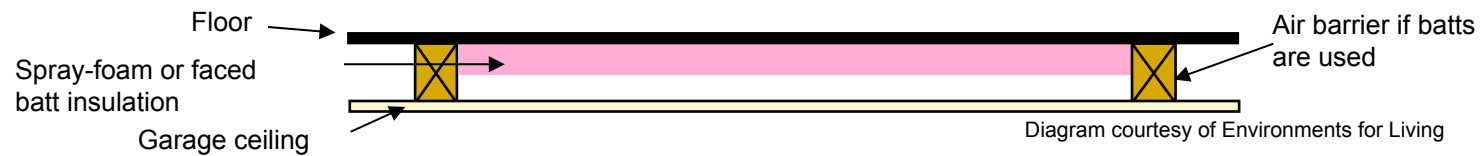
Figure 3.3 - Alignment of insulation and air barrier at garage ceiling with spray foam or faced batt insulation
