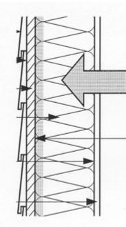
Warm, moist air moves from the interior toward the exterior in a heating climate
