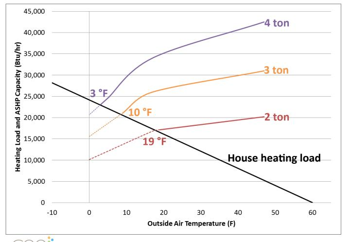
The OAT for the systems to switch to back up: 4 ton ~3 F 3 ton ~10 F 2 ton ~19F
